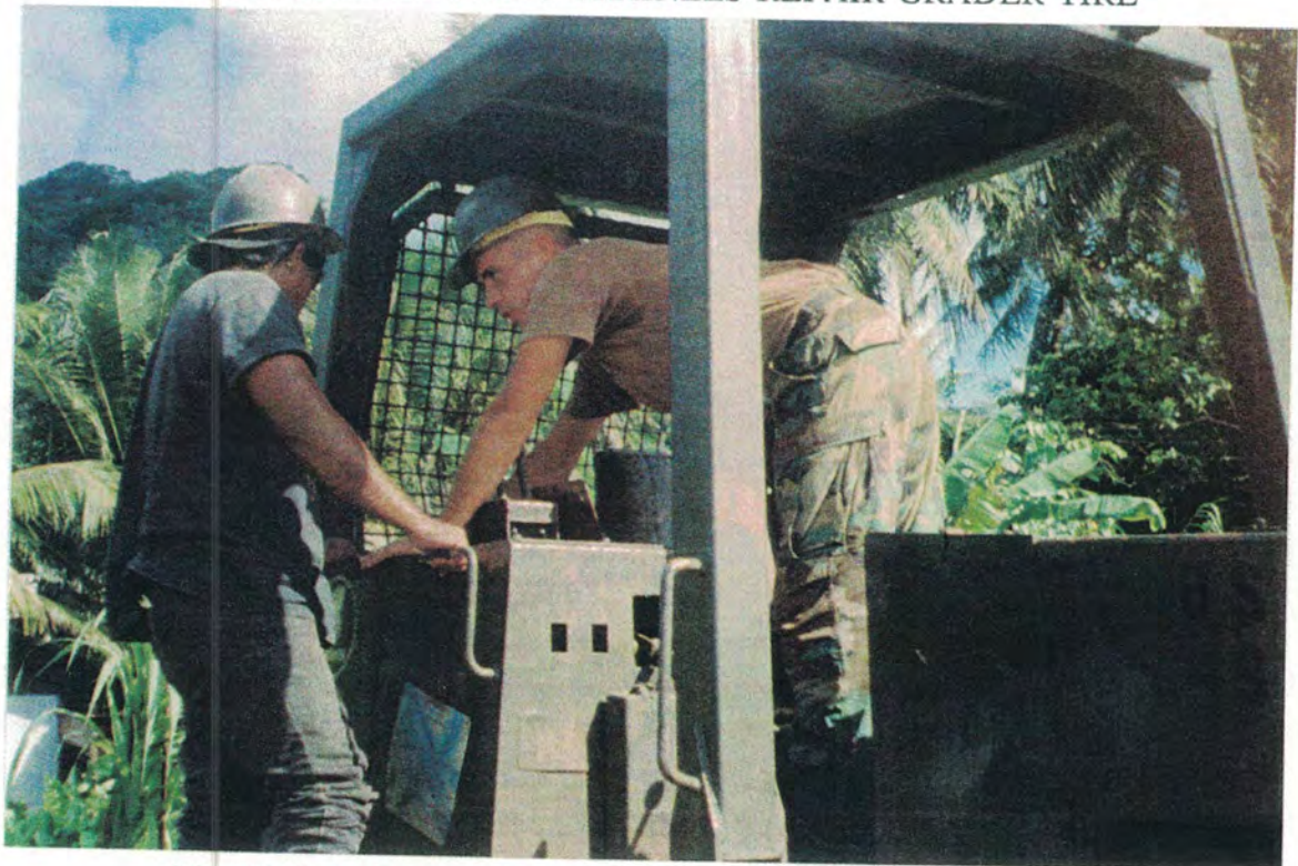
SOLDIER AND TRAINEE PERFORM PMCS ON BULLDOZER
